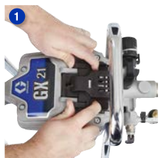
Slide & lift open access door
